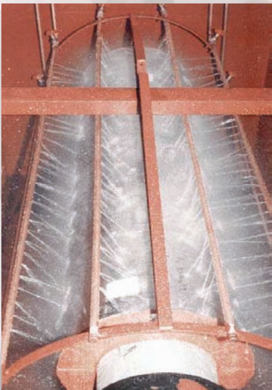
Water spray testing to demonstrate compliance with specification requirements regarding ingress of water and drainage capabilities
