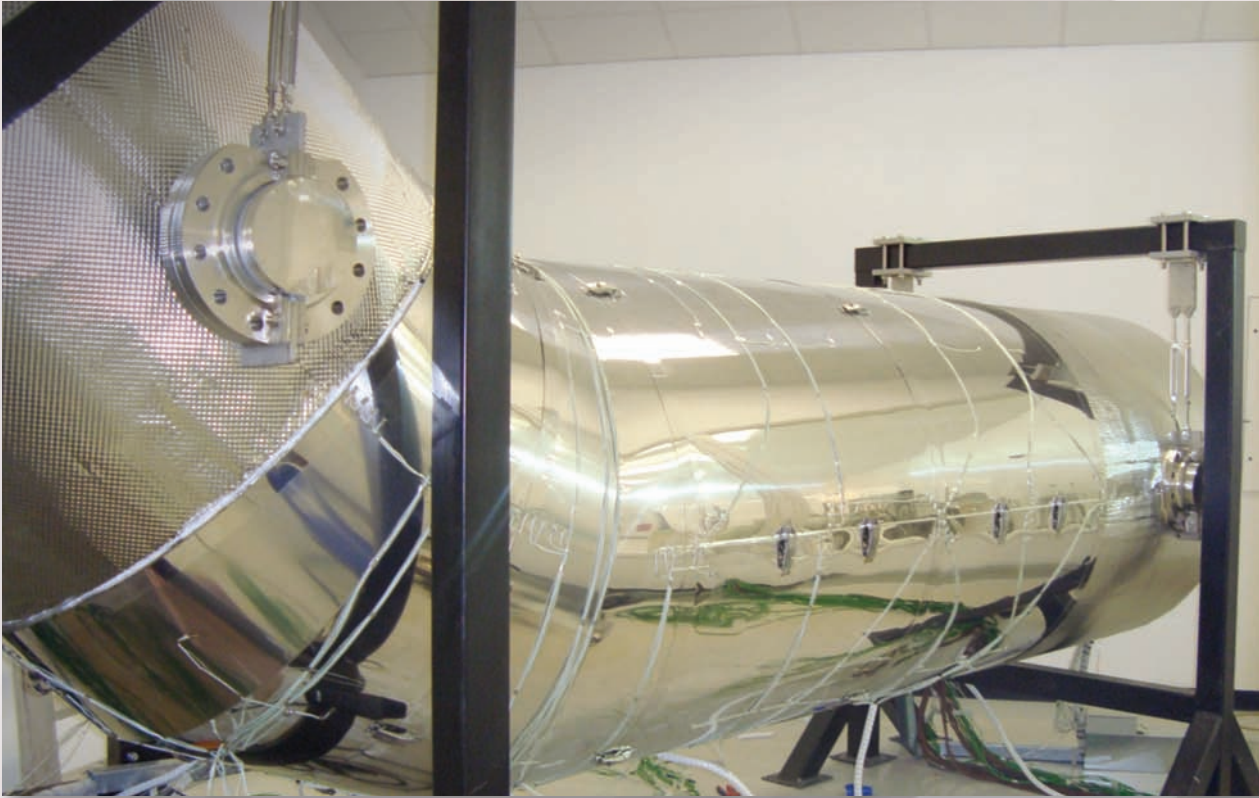
Thermal testing can be carried out on a 30 inch diameter pipe rig to represent a typical Primary Circuit Pipe.
